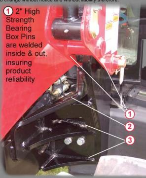
KMW Mounting Brackets are Engineered and Tested for Heavy Duty/Long Life
