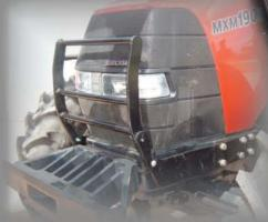
**Custom Fit Grill Guard Provides Tractor Front Protection**
